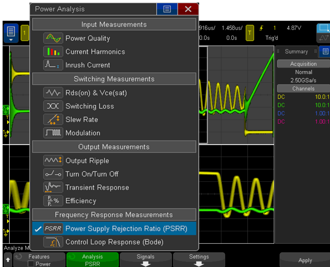
Figure 1. Power supply characterization measurements available in Keysight's InfiniiVision X-Series oscilloscopes.
