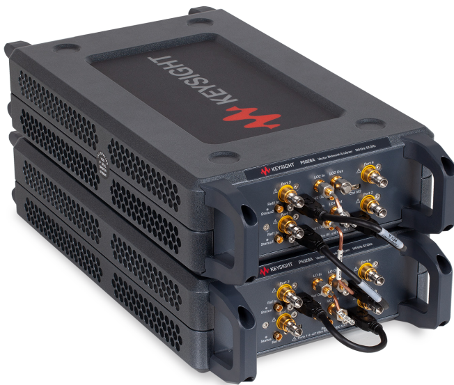
Figure 2. Eight-port, 53 GHz VNA made of two Keysight P5028 USB VNAs
