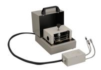
This 16008B test fixture can be used with the B2985A/87A to measure surface or volume resistivity of insulation materials. Three kinds of electrodes (diameter: 26 mm/50 mm/76 mm) are available to meet various insulation measurement standards such as ASTM D-257. The 50 mm diameter electrode is furnished with the 16008B as standard.
