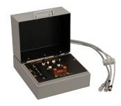
This 16339A test fixture can be used with the B2985A/87A to measure SMD, lead and various type of devices.
