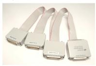
This adapter is required to use the multiple units of the B2901A/02A/11A/12A with EasyEXPERT group+software. The adapter has 4 Dsub25 connectors, which enables you to connect up to 4 units of the B2901A/02A/11A/12A and to control them through EasyEXPERT group+software.
