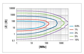
Figure 2. Measurement Time: Mode 2, Oscillator Level = 1 dBm, Averaging Factor < 8, Temperature Deviation  $\leq$  5 °C
