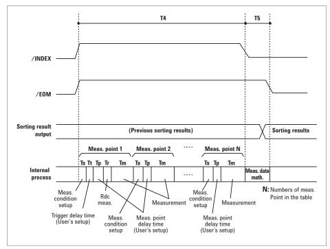
Figure 9. Measurement time T4 for list measurement
