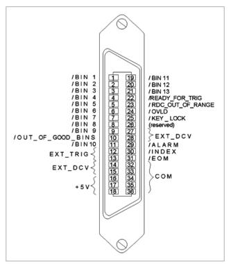
Figure 11. Pin assignment
