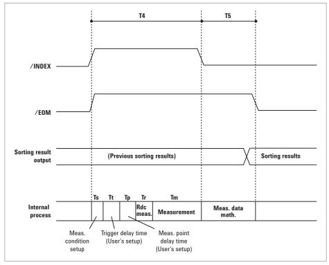
*Figure 8. Measurement time T4 for single point measurement*
