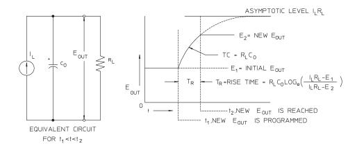
Figure 7-8. Speed of Response - Programming Up (Full Load)
