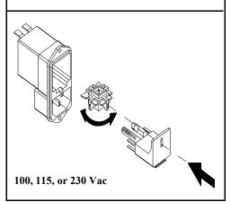
Replace the power-line voltage selector and the fuse-holder assembly in the rear panel.
