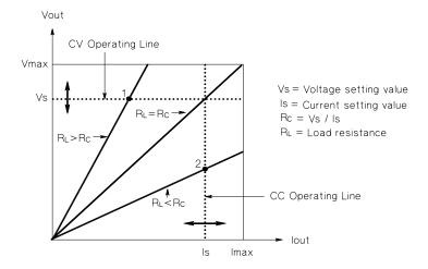
Figure 7-5. Output Characteristics
