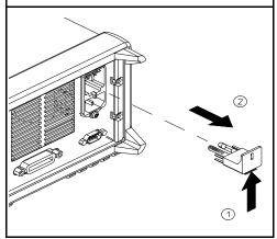
*Install the correct line fuse.* Remove the power-line voltage selector from the power-line module.
