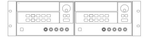
To rack mount two instrument of the same depth side-by-side, order lock-link kit 5061-9694 and flange kit 5063-9214.
