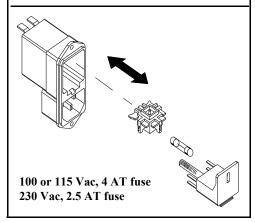
Rotate the power-line voltage selector until the correct voltage appears.
