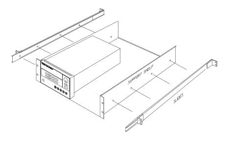
To install two instruments in a sliding support shelf, order support shelf 5063-9256, and slide kit 1494-0015.
