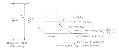
Figure 7-9. Speed of Response - Programming Down
