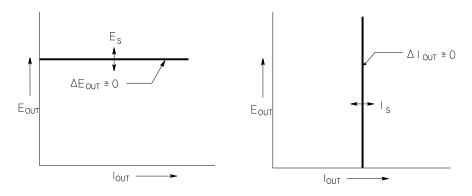
Figure 7-3. Ideal Constant Voltage Power Supply
