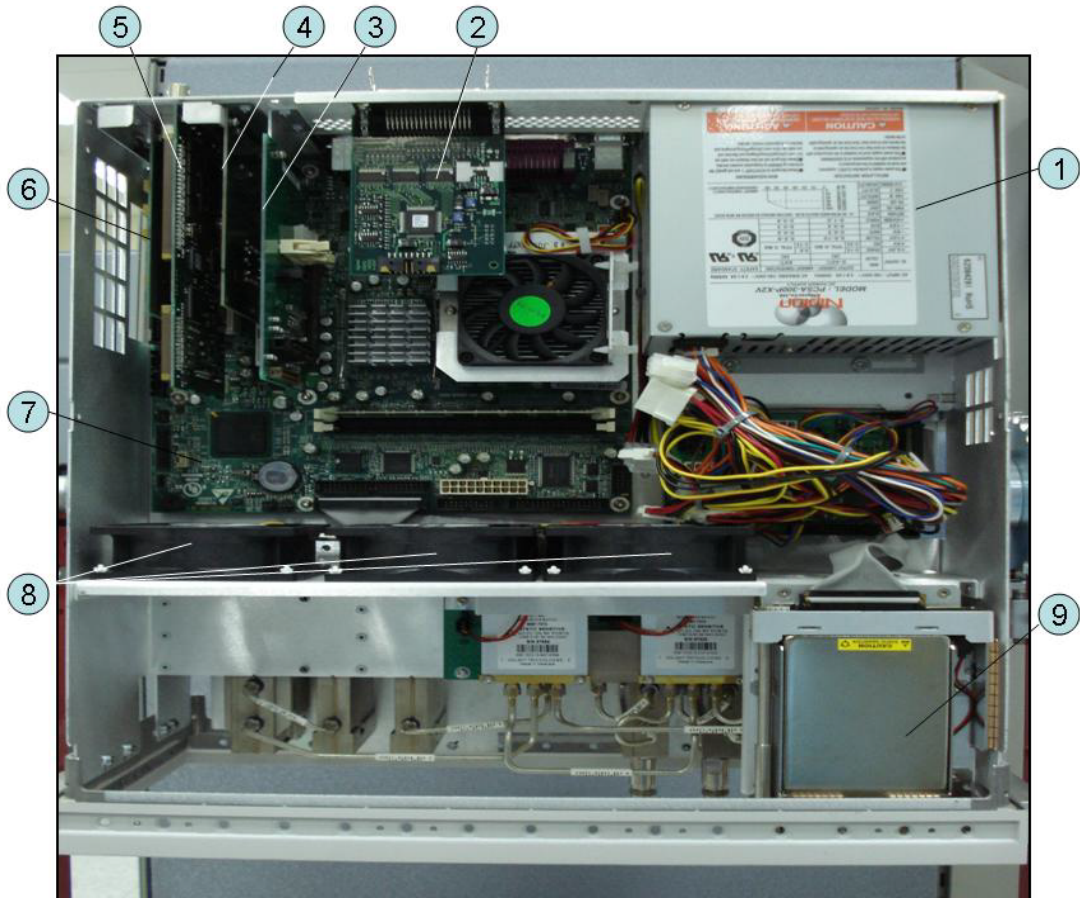
Figure 5-1 Top View (Major Assemblies) (Serial number prefix MY461 or SG461)
