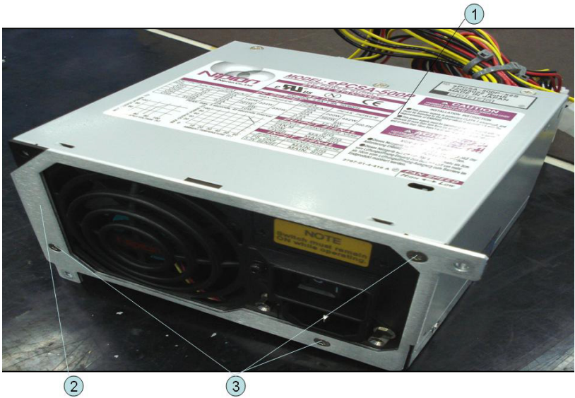
Figure 5-45 Power Supply (Over 8.5 GHz Options) Assembly
