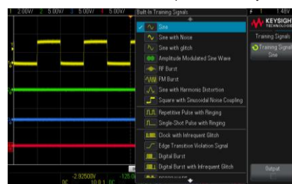
Built-in help and training signals
