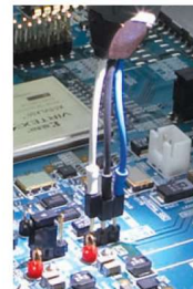
Solder-in tips N2750A with N2777A
