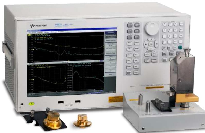
Applicable measurement instruments: E4991B (Option E4991B-002) <sup>3</sup>
